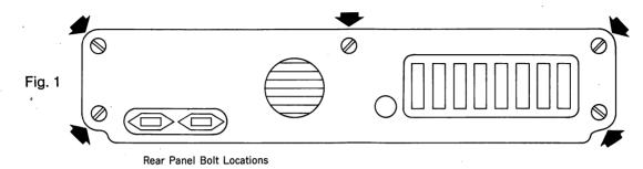
(From the front of the computer, grasp the left and right sides of the cabinet and pull toward you. The cover should slide without too much resistance.
