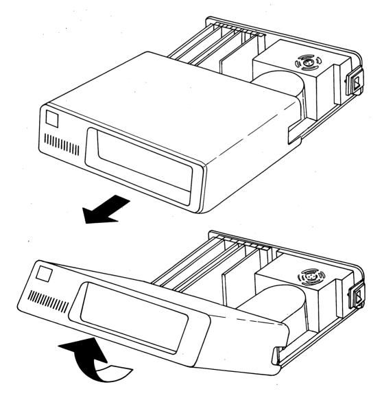
$\ast$  If the cover doesn't slide, check for snags between the cover and cables.
