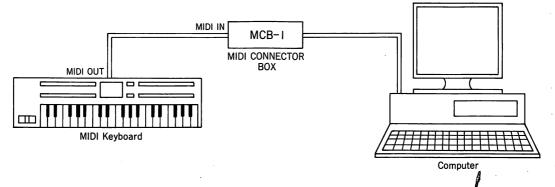
\* The sound source in the LAPC-I can be sounded even without using software, if an external keyboard is used for performance. When software is to be used, set THRU in the MIDI interface section to "ON" by means of the software. When THRU is not ON, performance information originating from the computer will generate sound, but an external keyboard will not produce sound. For details, refer to the manual for the software used.
