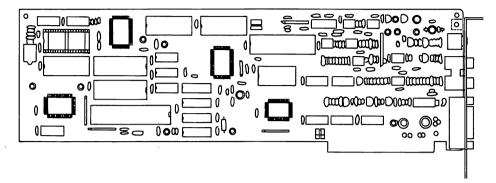
()Align the card edge connector over the connector slot and push the LAPC-I board into the slot.
