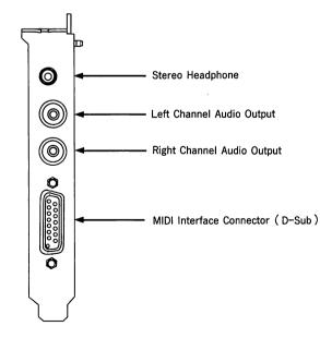
(i)Connect the MIDI connector box MCB-1 to the MIDI interface Connector. This box provides the connectors for attaching MIDI equipped keyboards and other devices to the LAPC-I card. This box also contains a metronome beeper.
