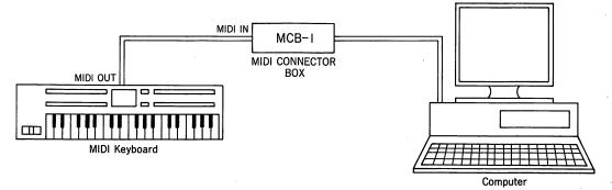
\* The sound source in the LAPC-I can be sounded even without using software, if an external keyboard is used for performance. When software is to be used, set THRU in the MIDI interface section to "ON" by means of the software. When THRU is not ON, performance information originating from the computer will generate sound, but an external keyboard will not produce sound. For details, refer to the manual for the software used.
