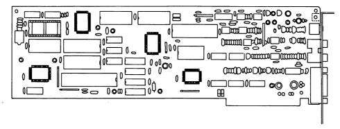
OAlign the card edge connector over the connector slot and push the LAPC-I board into the slot. Secure the board into the slot with the retaining screw.
