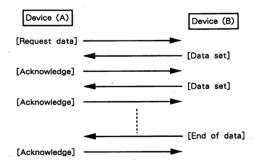
• Error occurs while device (A) is receiving data from device (B).
