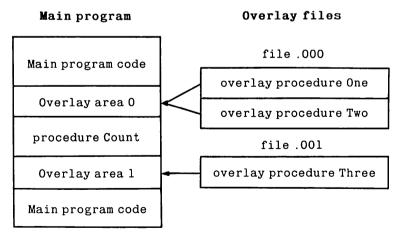
Figure 18-4: Multiple Overlay Files
