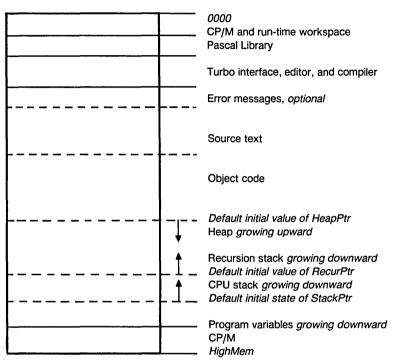
Figure 22-7: Memory map during execution in direct mode
