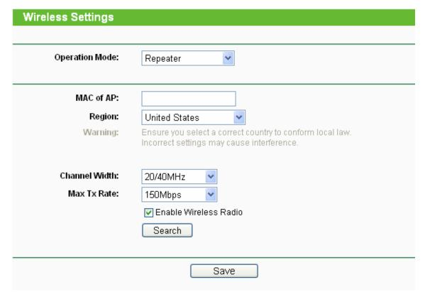
Figure 4-11 Wireless Settings in Repeater mode
