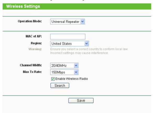
Figure 4-12 Wireless Settings in Universal Repeater mode
