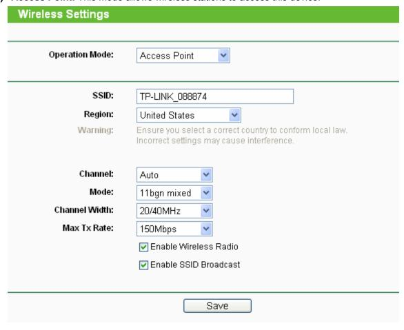
Figure 4-8 Wireless Settings in Access Point mode
