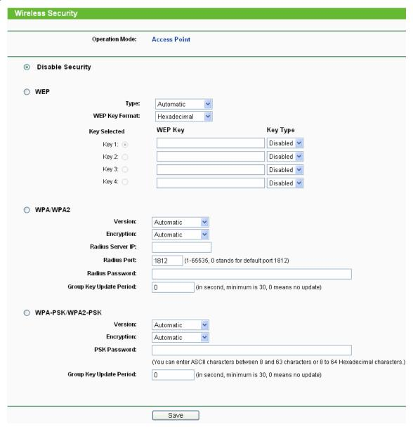
Figure 4-14 Wireless Security - Access Point
