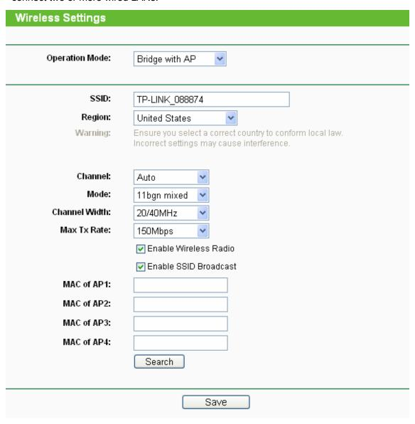
Figure 4-13 Wireless Settings in Bridge with AP mode
