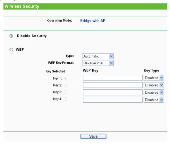
Figure 4-19 Wireless Security – Bridge with AP
