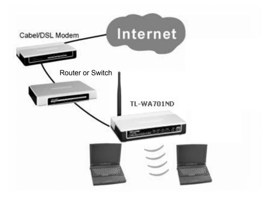
Figure 2-1 The Example of Infrastructure Network Incorporating the TL-WA701ND
