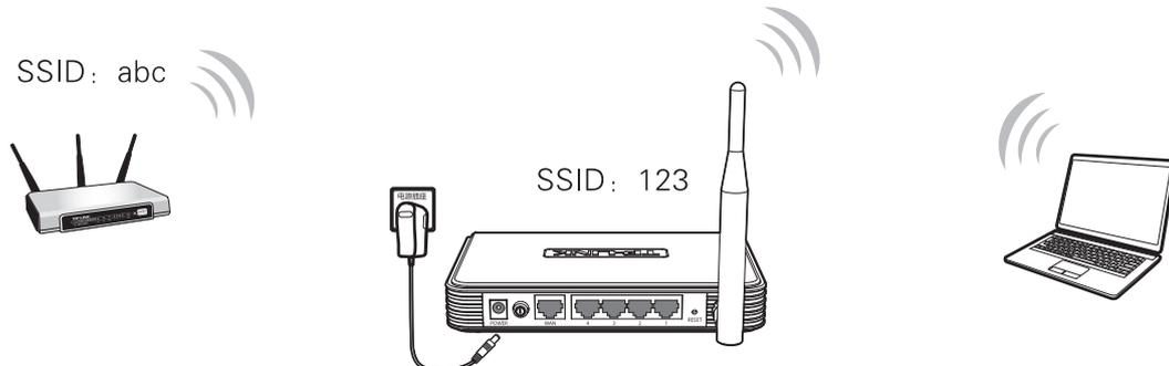
Figure 2-4 Hardware Installation of the TL-WR743ND in AP Bridge mode
