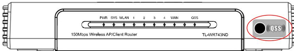
Step 2: Press and hold the QSS button of the adapter directly for 2 or 3 seconds.
