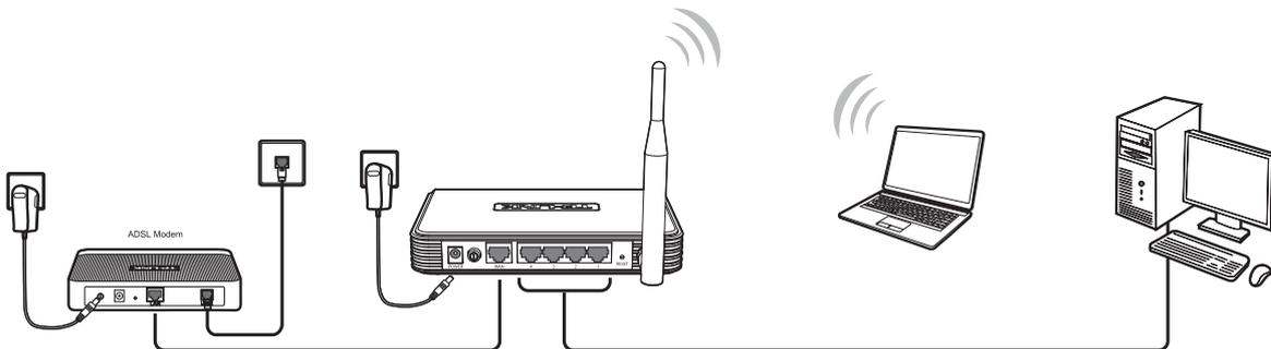
Figure 2-2 Hardware Installation of the TL-WR743ND in AP Router mode
