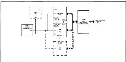
Figure 5. iAPX 186/20, 188/20 System Configuration
