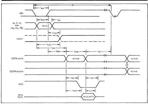
FIGURE 5. READ CYCLE TIMING
