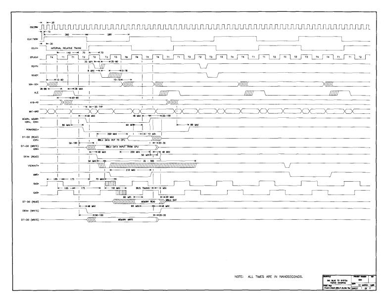
Figure 3. Big Blue to System Timing (1 of 2)
