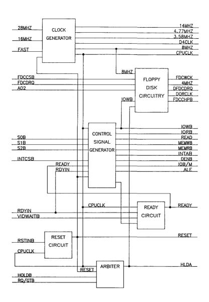
Figure 5. Timing Control Generator Block Diagram
