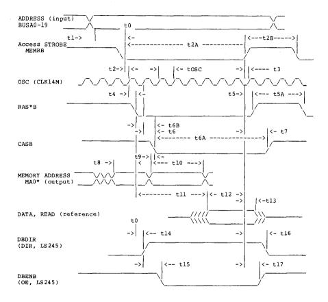
Figure 1. MEMORY TIMING PARAMETERS, READ
