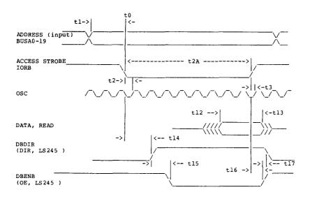
Figure 3. I/O CHIP SELECT PARAMETERS, READ
