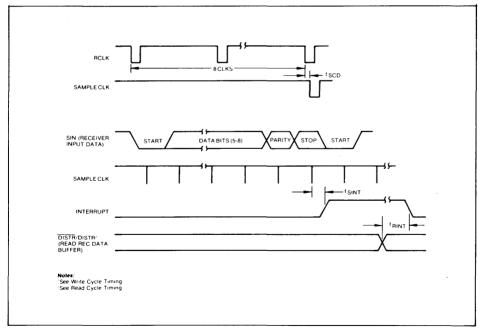
FIGURE 8. RECEIVER TIMING
