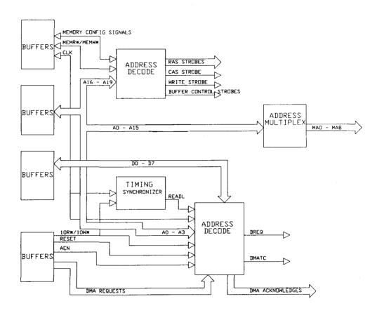
Figure 7. DMA/Memory Controller Chip Block Diagram
