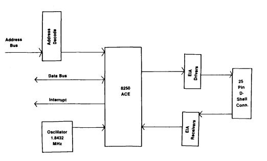
Figure 1. Block Diagram for the RS-232 Adapter.
