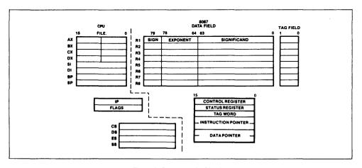
Figure 3. CPU+8087 Architecture
