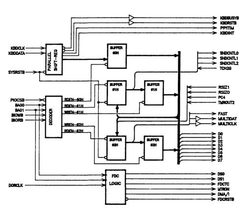
Figure 9. Keyboard Interface Block Diagram
