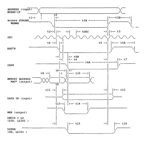
Figure 2. MEMORY TIMING PARAMETERS, WRITE
