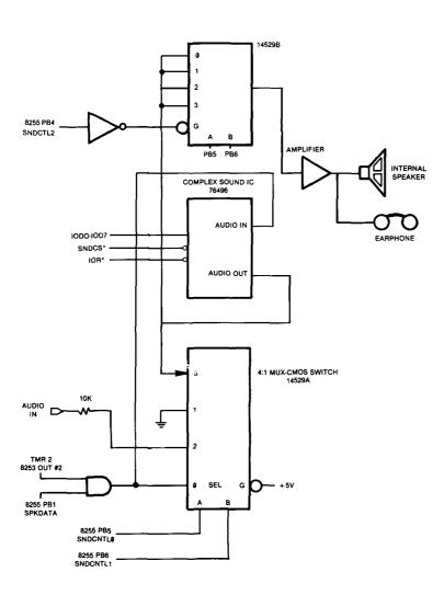
Figure 8. Sound Functional Block Diagram
