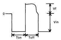
Collector Voltage Waveform
