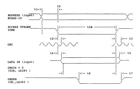
Figure 4. I/O CHIP SELECT PARAMETERS, WRITE
