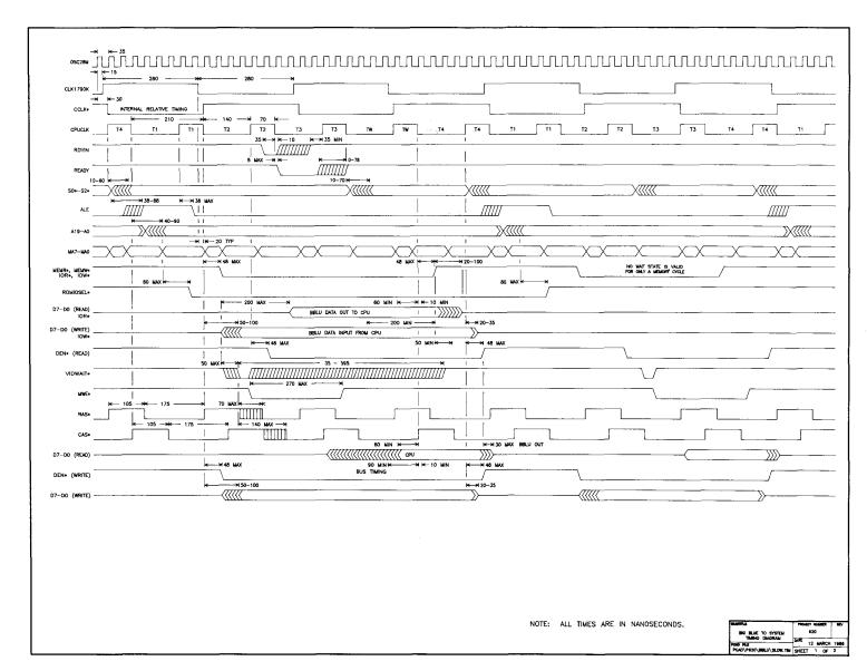
Figure 3. Big Blue to System Timing (2 of 2)
