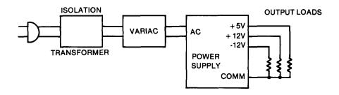
Figure 1 Test Setup
