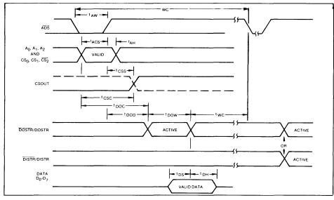
FIGURE 6. WRITE CYCLE TIMING
