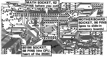
image of it. That 68-pin square will be to lower left rather than lower right as the picture shows, and the triple row of 96 pins to the left (right in picture). Our work will be done on the double row at center, 62 pins in two rows of 31. Note that I have numbered 61 and 62; the top row goes 61, 59, etc. down to 1 and the bottom row is 62 to 2.
