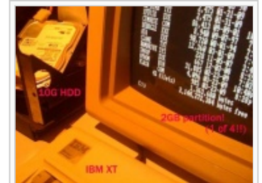
XTIDE controller on an IBM XT, running DOS 6.22 resulting in 8.4GB of total storage across multiple 2GB partitions; the maximum allowed with this OS.
