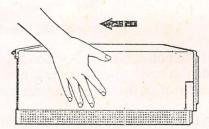
Figure 2-6. Slide the cover into place.
