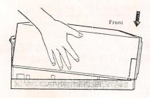
Figure 2-5. Replacing the top cover.
