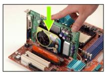
**3.** .Insert a PCIE graphics card into PCIEXP1 slot.
