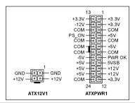
**Note:** It is recommended to connect to a power with 350W, 20A +5VDC capacity at least for heavily loaded system, and a 2A +5VSB capacity at least for supporting wake-up features.
