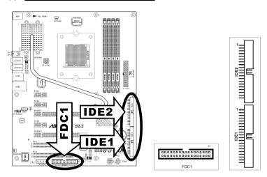
The FDC1 connector connects up to two floppy drives with a 34-wire, 2-connector floppy cable. Connect the single end at the longer length of ribbon cable to the FDC1 on the board, the two connectors on the other end to the floppy disk drives connector. Generally you need only one floppy disk drive in your system.
