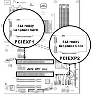
**SLI Mode:** Insert 2 identical SLI-ready graphics cards into PCIEXP1 and PCIEXP2 slots.
