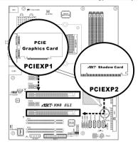
**Normal Mode:** Insert your PCIE graphics card into PCIEXP1 slot, and the ABIT Shadow Card into PCIEXP2 Slot.
