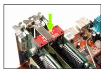
**6.** Insert the SLI bracket into the bracket slot between the graphics cards. Secure the SLI bracket and the graphics cards to the chassis with screws.
