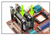
1. Insert the two graphics cards into PCIEXP1 and PCIEXP2 slots on the motherboard.
