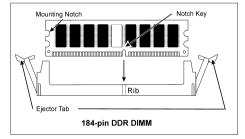
5. To remove the DIMM modules, push the two ejector tabs on the slot outward simultaneously, and then pull out the DIMM module.
