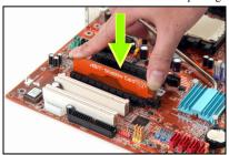
Insert ABIT Shadow Card into PCIEXP2 slot.
