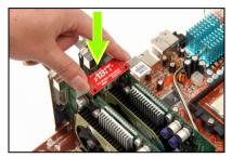
**4.** Insert the SLI Bridge Connector into the SLI goldfingers on each graphics card.
