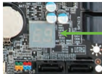
Debug LED with CPU Temperature Monitor
