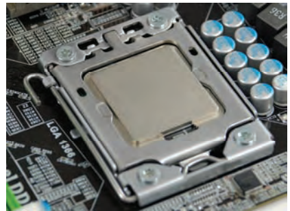
Align notches with notches on the CPU
