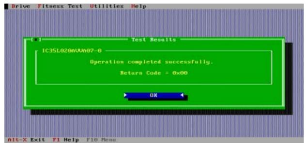
The screen above shows the conclusion of a test. In this case, the drive passed the DFT testing.
