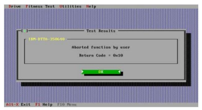
This says that testing has <u>not</u> been completed, and is not a statement of either pass or fail. Testing must be restarted and run to completion in order to assess if there is a problem with the drive. The return code 0x10 is not an error.
