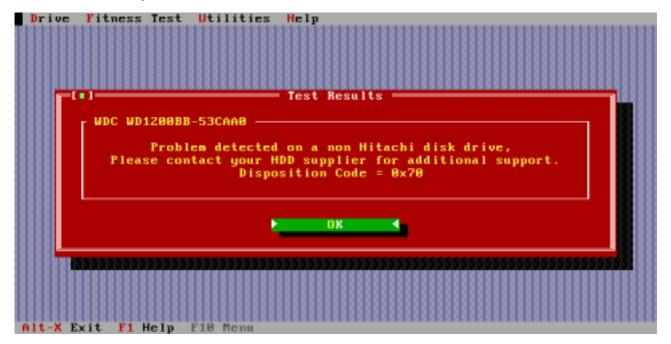
Running the Erase Disk, Erase MBR functions on non-Hitachi/IBM disk drives is not supported by DFT. The screen below will be displayed if you attempt to run any of these functions on a non-IBM hard disk drive.
