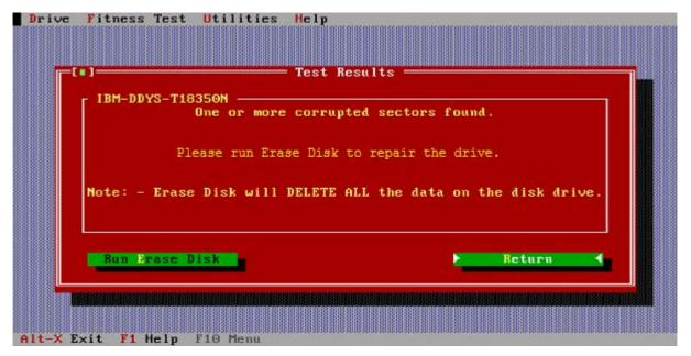
In most cases when DFT reports a media error this is because the data in a sector cannot be read due to corruption. These corrupted sectors can be recovered by being re-written, see options below.
