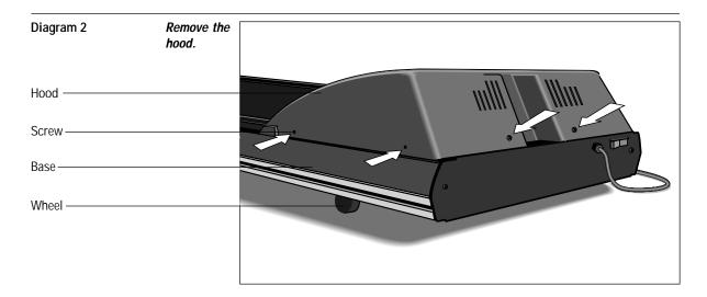
Remove the treadmill's hood using a phillips head screwdriver. Unscrew all six screws and set them aside. See Diagram 2. Grasp both sides of the hood with your hands and pull up to remove the hood from the base.
