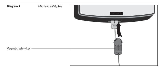
Before you can begin a workout, you must insert the magnetic safety key into the electronic console as shown in Diagram 9. The treadmill's running belt will not move unless the safety key is inserted and secure inside the electronic console. To prevent unauthorized use of the treadmill, store the safety key in a safe place.
