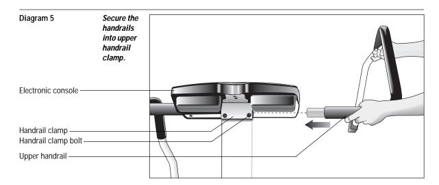
9. Insert the upper end of a handrail into the upper handrail clamp. Using one hand, apply pressure on the portion of the handrail going into the clamp while, with the other hand, lift and lower the base of the handrail. This rotating motion helps move the handrail into place. The handrail is properly positioned when the black foam wrap touches the clamp as shown in Diagram 5. Repeat this step for the other handrail.
