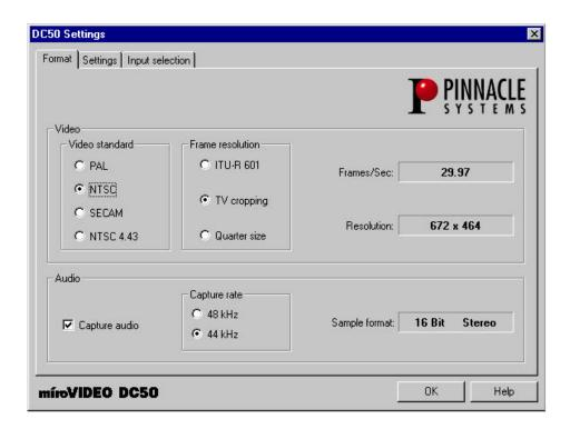
If you want to create a new project with other capture format settings you should load the appropriate Preset. This is the only way to keep capture format and Premiere playback format the same.
