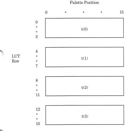
The hardware cycles through the LUT every second, so each quarter of the LUT is active for <sup>1</sup>/<sub>4</sub> of each second. The cycling mechanism produces blinking. The following examples show the details of how you can produce several different blinking effects by setting different values in the LUT.
