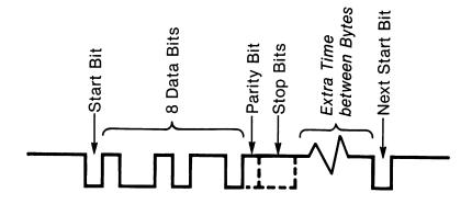
Figure 7-1. The transmission of one byte of serial data.
