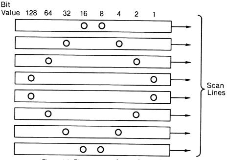
Figure 4-3. Bit patterns to form a diamond.
