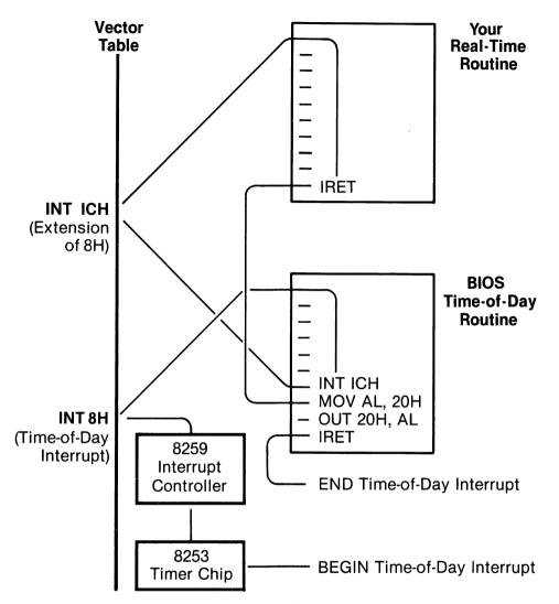
Figure 2-3. Extending the timer interrupt.
