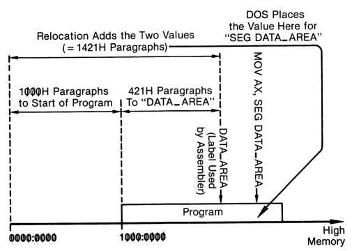
Figure 1-6. Relocation of the memory position of "DATA\_AREA".
