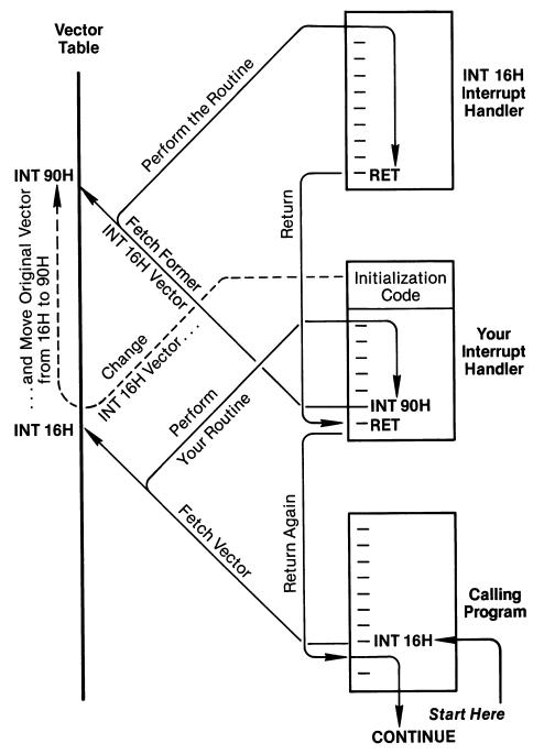
Figure 1-3. Adding on to an existing interrupt.
