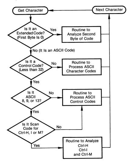
Figure 3-3. Flow Chart For A General Input Routine.
