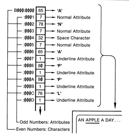
Figure 4-2. Memory mapping on the monochrome adaptor.
