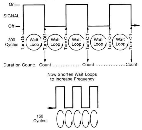
Figure 2-4. Producing sound by the 8255 chip.
