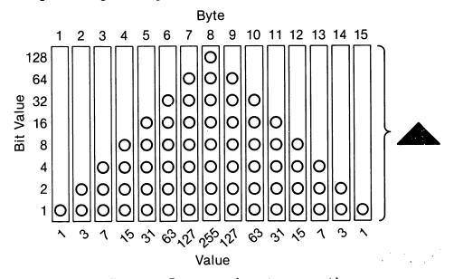
Figure 6-1. Bit patterns that print a pyramid.
