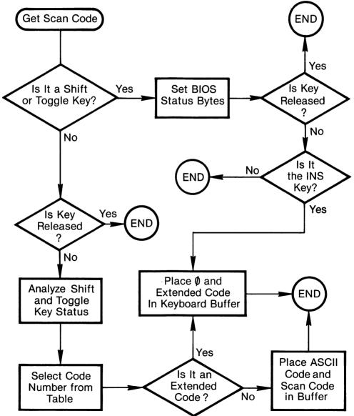
Figure 3-4. The Keyboard Interrupt.
