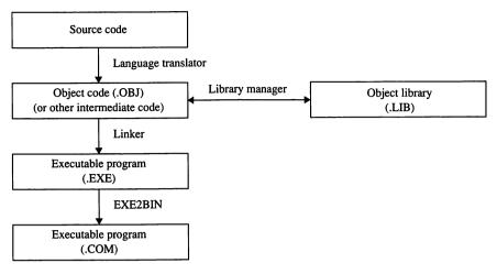
**Figure 19-3.** Building an executable program. By convention, object filenames use the .OBJ extension; object libraries use .LIB; executable files use .EXE or .COM.
