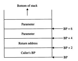
Figure 8-4. The stack after register BP is initialized.
