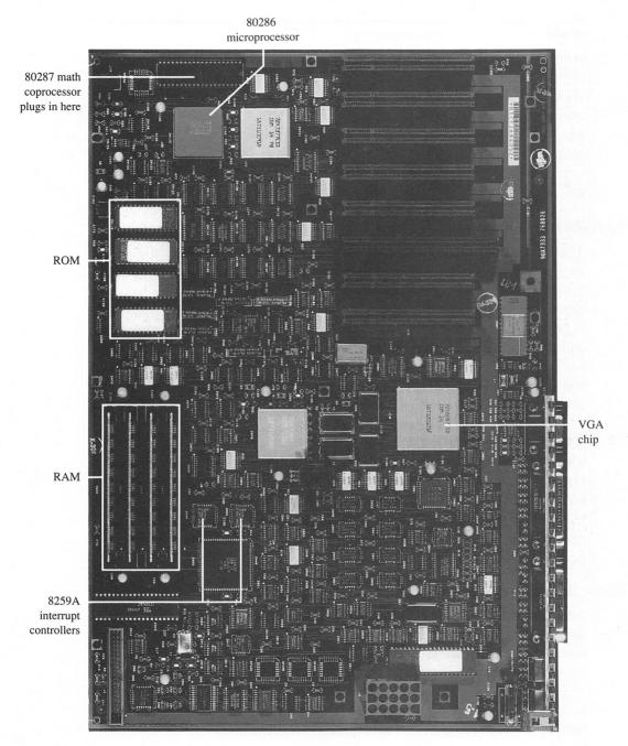
Figure 1-3. The PS/2 Model 60 system board.
