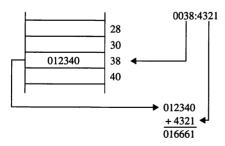
**Figure 2-4.** Decoding an 80286 protected-mode segmented address. The segment selector 38H indicates an entry in a segment descriptor table. The segment descriptor contains a 24-bit segment base address which is added to the offset 4321H to give the 24-bit physical address 016661H.
