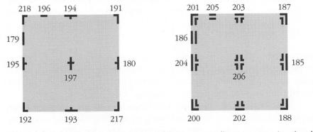
**Figure C-6.** The box-drawing characters and their corresponding (continued) ASCII codes.
