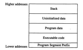
Figure 19-1. Memory usage in a typical DOS program.
