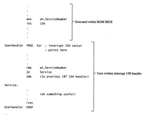
Figure 12-12. How the ROM BIOS hooks can be used.
