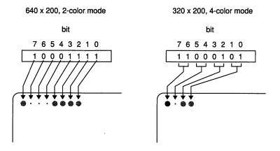
Figure 4-13. Pixel mapping in CGA-compatible graphics modes.
