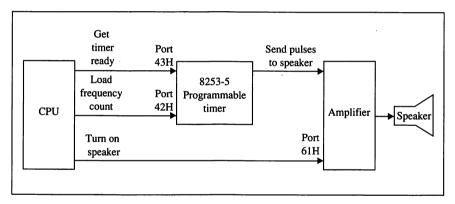
Figure 7-3. How sound frequencies are generated through the system timer and speaker.
