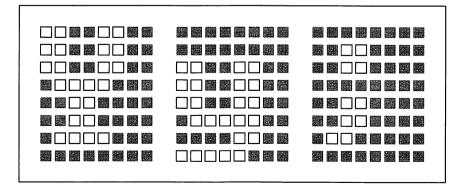
Figure C-3. The dot pattern of three characters in an  $8 \times 8$  character box.
