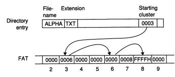
Figure 5-14. Disk-space allocation using the FAT.
