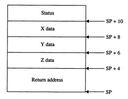
Figure 12-9. Pointing-device data packet.
