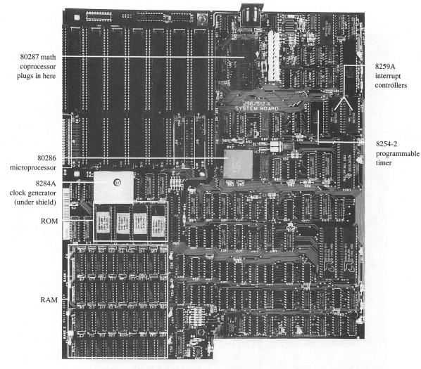
Figure 1-2. The PC/AT system board.
