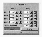
videotape. Your computer must have a VISCA compatible VCR attached and have a SNAPplus or Video Blaster card installed in order to use this feature.
