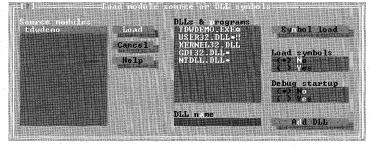
The Source Modules list box displays all the source modules contained in the currently loaded executable file. The DLLs & Programs list box displays all the .DLL and .EXE files that are currently loaded by Windows. (If you're running TDW, the list also displays all loaded .DRV and .FON files.) Check Show Full Name Paths to view the directory and path to your source modules.
