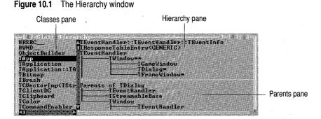
The Hierarchy window displays the heritage of object-oriented program classes. The window is composed of two or three panes, depending on whether or not your program uses multiple inheritance.
