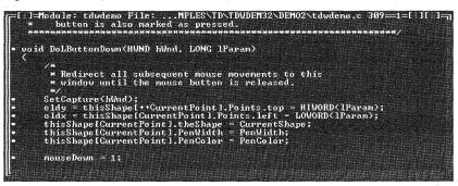
When you open the Module window, the title bar displays the name of the currently loaded module, the name of the current source file, and the cursor's line number.
