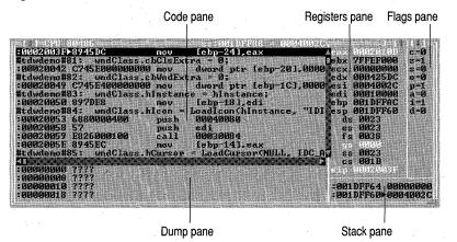
From within the Code, Dump, and Stack pane, it's possible to scroll outside the current protected-mode segment, even though the operating system marks these as invalid addresses for your program. Because of this, the CPU window displays question marks for any addresses referenced outside the current protected-mode segment.
