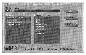
The Files list box displays the files in the currently selected directory. By entering a file mask into the File Name input box (such as \*.*EXE*), you can specify which files should be listed. You can also use the File Name input box to change disk drives.
