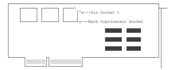
WARNING: Incorrect installation of a math coprocessor can damage the coprocessor, the CPU board, and/or the main logic board.
