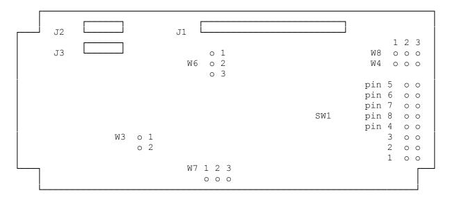
The 25-1029 /A/B Use the Western Digital hardcard controller stock # WD1002A-WX1 and comes configured for use in the Tandy 1000 /A/SX/TX. The jumpers should be confirmed correct for the computer it is to be installed in.
