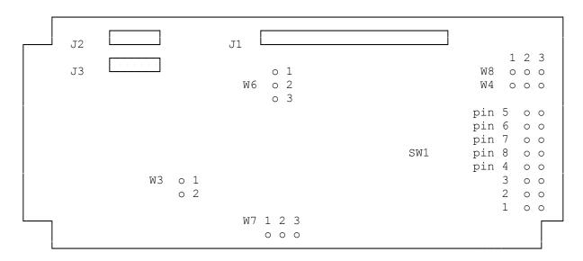
The 25-1032A /B all use the Western Digital hardcard controller stock # (WD1002A-WX1) and comes configured for use in the Tandy 1000 /A /SX /TX. The jumpers should be confirmed correct for the computer it is to be installed in.
