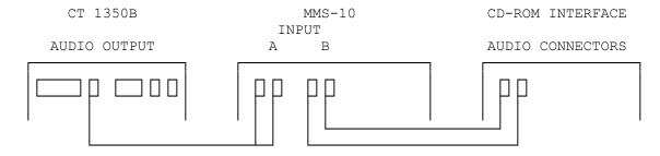
Note: Although the CD-ROM is connected to Input B, and the CT 1350B is connected to Input A on the MMS-10, this is not a requirement for operations. The user is free to select any Input Channel for the CD-ROM Interface and CT 1350B.
