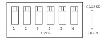
Dip switch settings: SWITCH SYMBOL OPEN CLOSE Interface 8-bit Parallel Serial Baud 1200 600 3 Paper Empty Enable Disable Impact High Low Self test Not App Applied Auto logic seek Applied Not applied
