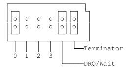
This CDR 1501 drive is capable of being daisy chained with up to three more CDR-1501 drives. Radio Shack does not sell a cable to support this configuration. The customer will have to find a 40 pin cable locally.
